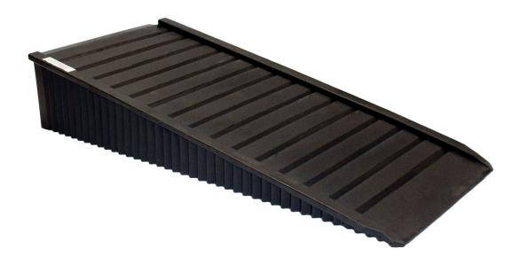
The ribbed, non-skid surface of this ramp allow for additional traction when loading drums with a hand truck. The 10 degree slope is easy to maneuver and the polyethylene construction won't rust or corrode. It has a strong 1,000 lb. handling capacity and is compatible with a variety of ENPAC products, including:
